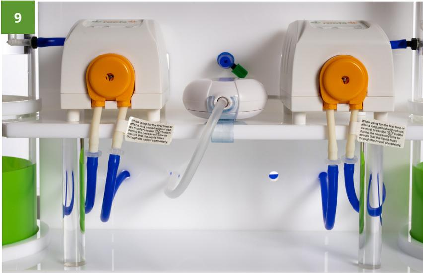
Once the pumps have been calibrated, connect the blue tube of the feed supply, maintaining the position shown in the picture.
