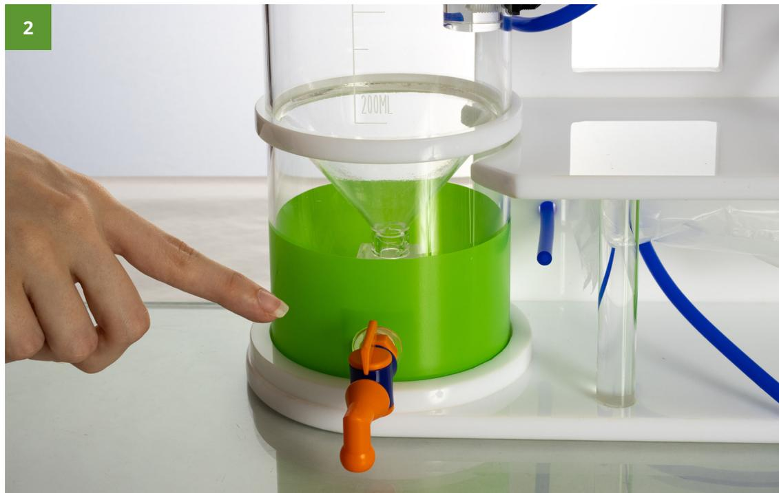
Position the reactor cylinders so that the outlet valve is in front position.
