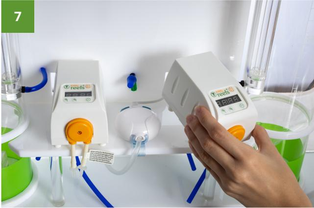
Place the Easyfeeder dosing pumps (Master and Slave) in their position. Calibrate the dosing pumps according to the instructions inside the box.
