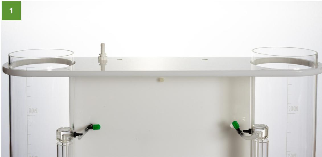
Unscrew the screws on the cylinder fixing plate and remove it.
